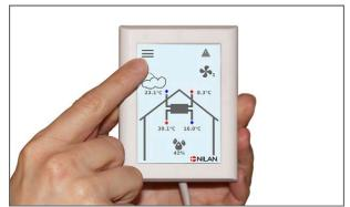
6. In the ALARM menu on the control panel, press the alarm symbol at the top right and reset the alarm here.
