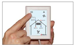
8. In the ALARM menu on the control panel, press the alarm symbol at the top right and reset the alarm here.
