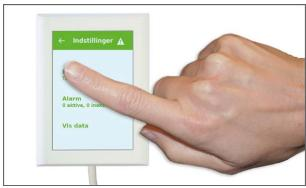
1. Before opening the door, switch the unit off on the control panel under OPERATION. This is situated in the main menu SETTINGS  $\frac{1}{2} \frac{1}{2} \frac{1$
