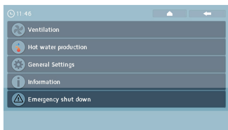
5. When the danger has passed and the ventilation can be used again, press "Emergency Stop Ventilation" once more.
