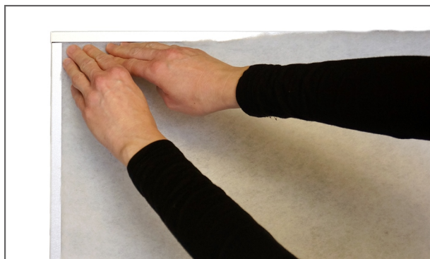
7. Press the filter sheet firmly in place and carefully push it to the sides of the filter frame. The filter is placed back in the unit with filter mat upward
