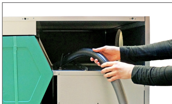
4. It is advisable that you vacuum the filter chambers for potential dirt and dust
