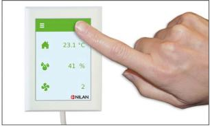
$6.\,Go\,View\,menu\,ALARMS$  on betjeningspanet and reset the alarm here
