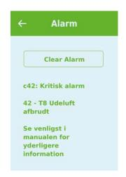
If the ventilation unit is faulty or an error occurs, there will be either a warning or an alarm. The icon will appear in the top right hand corner in the menu bar.
