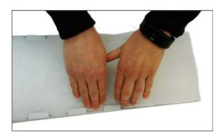
7. Press the filter sheet firmly in place and carefully push it to the sides of the filter frame.
