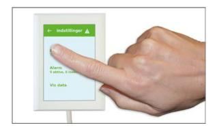
1. Before opening the door, switch the unit off on the control panel under OPERATION.  $\label{eq:control}$
