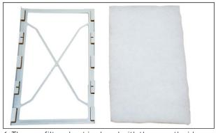
6. The new filter sheet is placed with the smooth side down in the filter frame.
