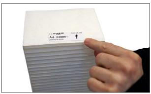
4. The new pollen filter must face the arrow away from the duct connections.
