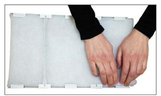
7. The filter sheet is clamped firmly in the filter frame and pushed well into the sides. The filter is again placed in the unit with the filter sheet facing upwards.
