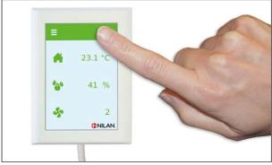
6. Turn on the unit again and press the ALARM icon to reset the warning.
