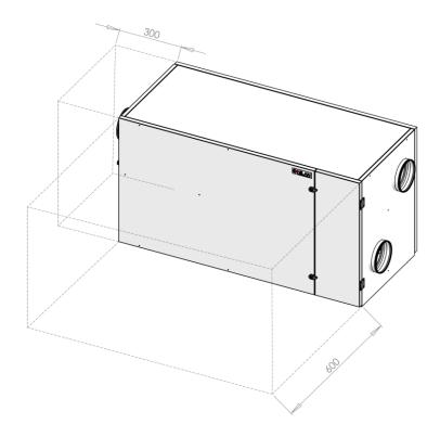
Figure 2: Mounting the Combi 300 Polar
