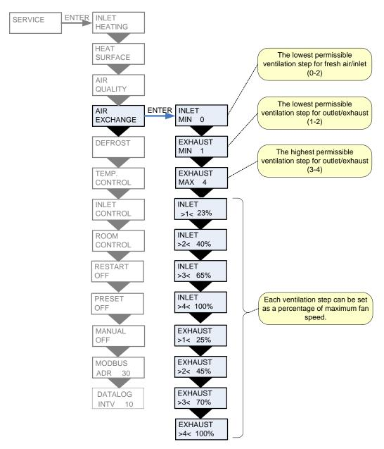
Figure 10: The "Air exchange" Menu
