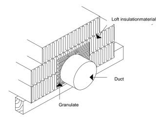
Figure 4: Insulation of ducting
