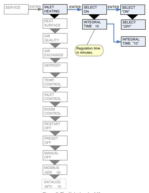
Figure 7: The "Inlet heating" Menu
