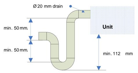
Figure 3: Condensation drain / water seal
