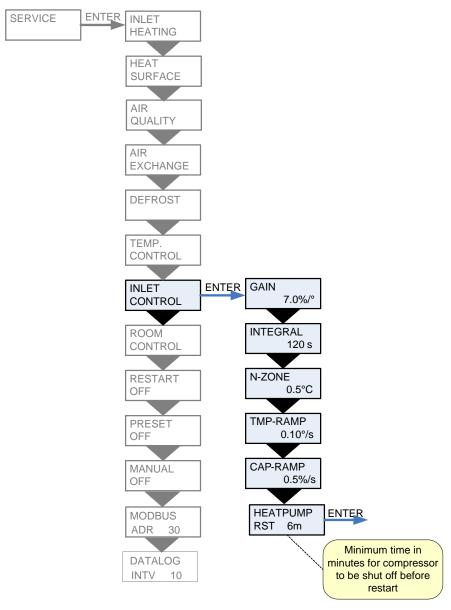
Figure 13: The "Inlet control" Menu
